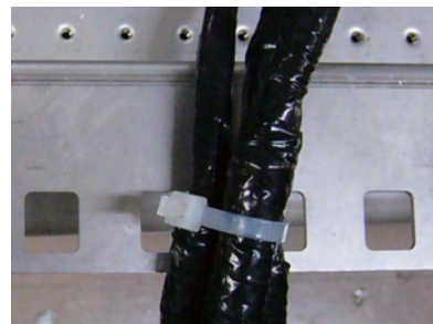
Fix cables to post with cable tie
